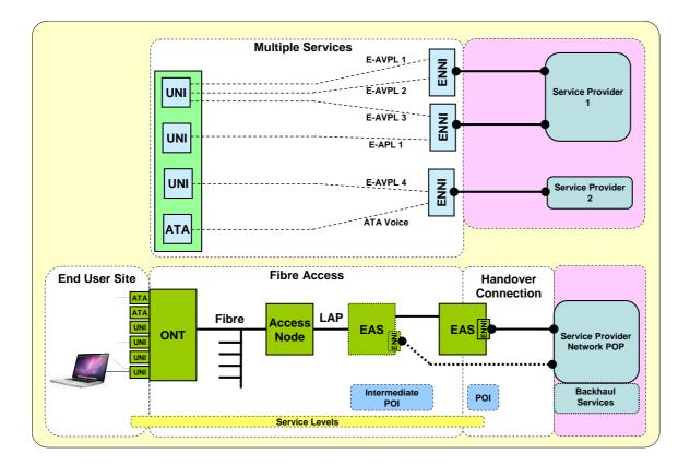
This is a generic diagram showing the standard configuration and service demarcation points. It is not intended to represent every situation or detailed physical architecture. The following points should be noted:
