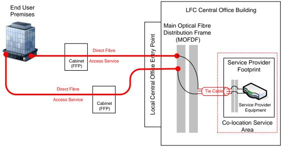
Single Central Office redundancy with separate diverse fibre, diverse access to End User Premises and diverse access to a separate OFDF at a single Central Office
