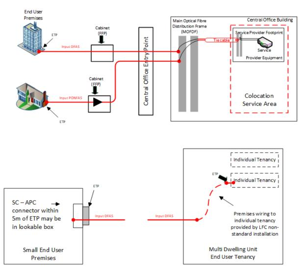
This is a generic diagram showing the standard configuration and service demarcation points. It is not intended to represent every situation or detailed physical architecture. The following points should be noted:
